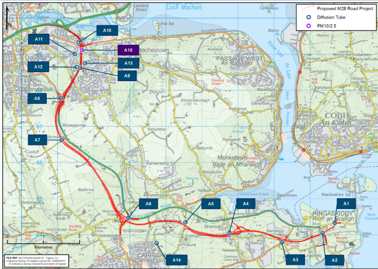
Figure 13.1: Baseline Air Quality Monitoring Locations
